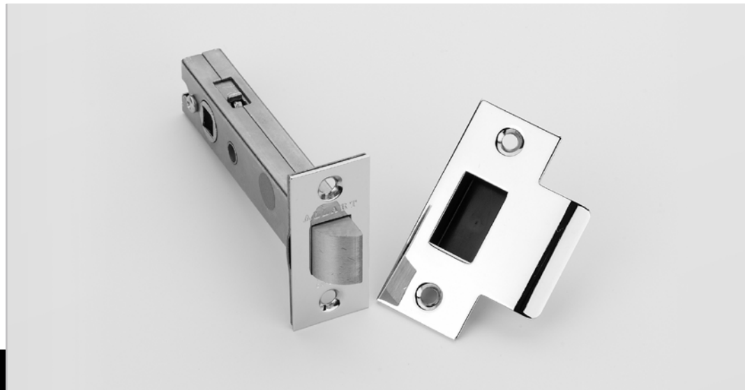
▲ 7500 (light springing - for use with unsprung regular Knob Sets & sprung Lever Sets) ▲ 7512 (heavy springing - for use with unsprung Lever Sets & unsprung heavy Knob Sets)
